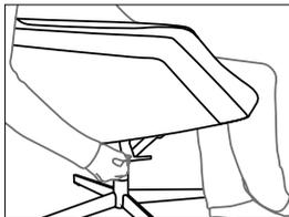
Pull left lever upwards → unlocks the back section
